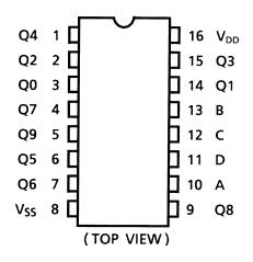
Note: xxxFN (JEDEC SOP) is not available in Japan. TC4028BP DIP16-P-300-2.54A TC4028BF SOP16-P-300-1.27A TC4028BFN SOL16-P-150-1.27 Weight DIP16-P-300-2.54A : 1.00 g (typ.) SOP16-P-300-1.27A : 0.18 g (typ.) SOL16-P-150-1.27 : 0.13 g (typ.)
